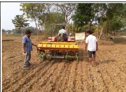
Line sowing of green gram by seed cum fertilizer drill
